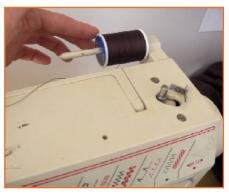
Step 1: This is where the thread goes. If you have a cap or stopper put it on after you put the thread on. Also put the side of the thread with the little cut to the back or bottom.
