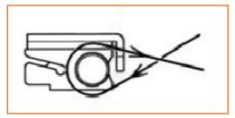
**Step 1:** • Place spool of thread on spool pin.
