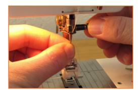
Step 4: Use your fingers initially and then your tool of choice to tighten the needle clamp screw. The tighter you can make this, the better. A loose clamp may leave the needle down in the fabric you are sewing.
