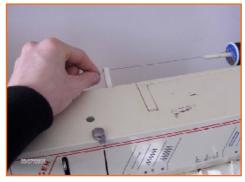
Allow the string to unwind and put it through this hoop. Mine can also snap in from the back but usually with older machines this is a hoop.
