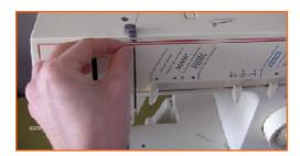
From the tension bring the thread up and from right to left put it through the hole here.
