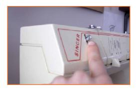
Step 5: Then bring it down from the take up lever into the coiled thread guide.
