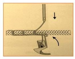
Step 2: • The needle moves up and comes out of the cloth and the unstitched portion of cloth is pushed forward to form a stitch.
