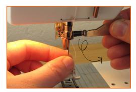
Hold the needle with your left hand Step 1: and undo the screw at the top of the needle with your right hand.
