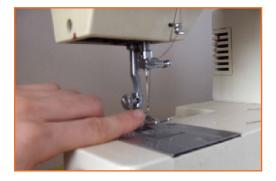
Step 7: Then thread the needle front to back or right to left depending on your machine. Pull enough thread through so that it does not pull out when the needle moves 5-10 inches.
