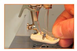
Step 5: Re-thread your needle, pushing the thread from front to back.
