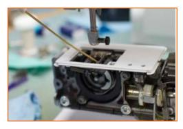
Check feed dogs: Remove the feed dog, clean the feed dogs. Try to pass a rag under them and with an old needle or narrow tool, remove the lint inside the feed channels. Put back the needle plate. If your machine is equipped with a FEED DROP, be sure the feeds are set at UP position. By turning the hand wheel (towards you), check to see if the feeds make their movement.
