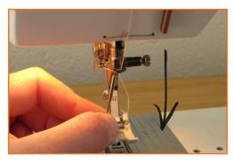
Remove the needle by pulling down and away from the needle clamp.
