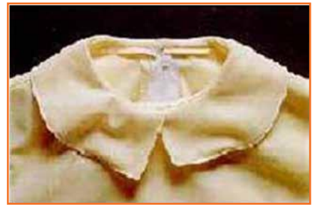
Fig.3.1.22(c): Interlining shrinking
