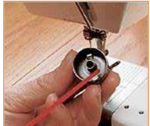
Fig.4.1.2: Cleaning the bobbin and case
