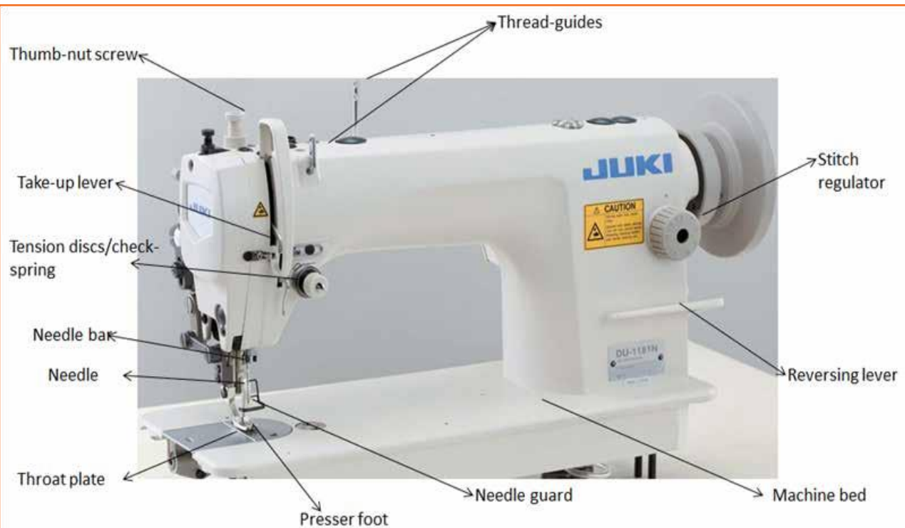
Fig.2.1.20: Parts of a Sewing Machine
