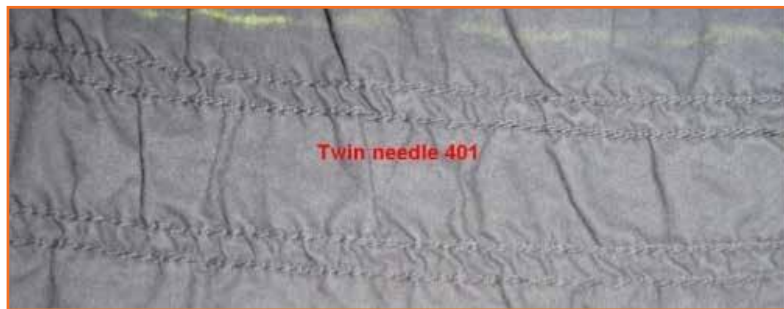
Fig.3.1.9: : Shrinkage pucker occurs during the
